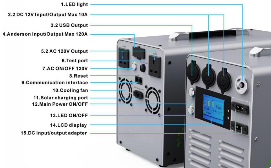
Figure 1. The main operation buttons/ports list
